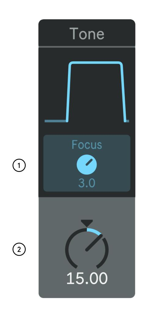
Tone [B] is a non-resonant lo/hi-cut filter with variable steepness, affecting the Delay B output signal. It is exactly the same as the Tone for Delay A.
