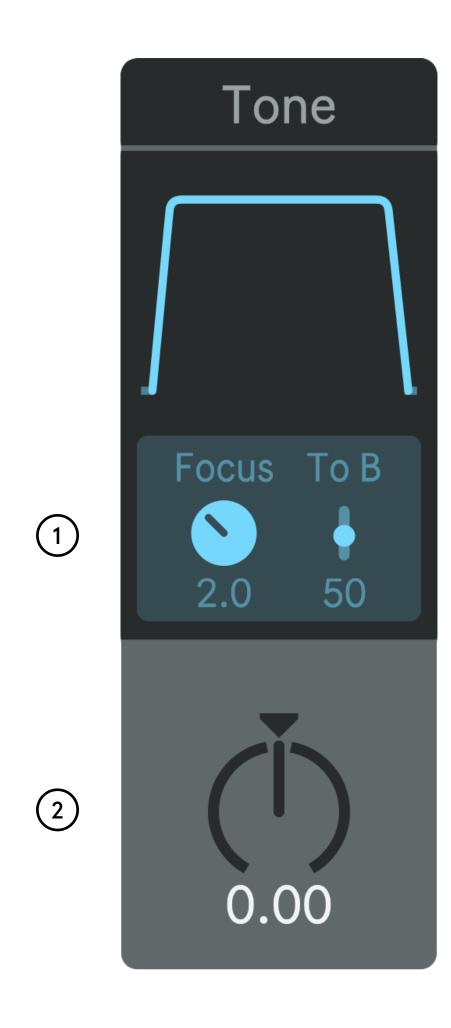
Tone [A] is a non-resonant lo/hi-cut filter with variable steepness, affecting the Delay A output signal.
