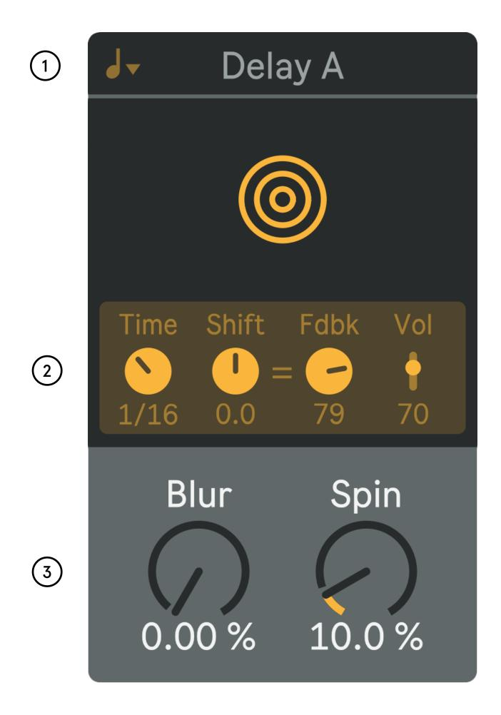
Delay A is a diffusing delay that can be pitch shifted and modulated. Delay A is in mono and can be sent to Delay B for further processing.
