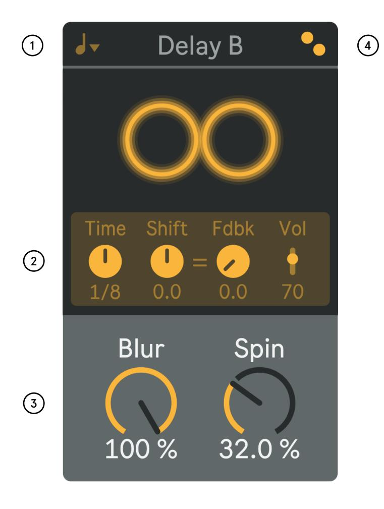
Delay B is a diffusing delay that can be pitch shifted and modulated, its controls are almost identical to Delay A. The only difference is that Delay B is in stereo.
